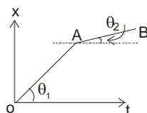
O to A velocity is constant i.e.  $V$ , also from A to B velocity is constant but  $\theta_2 < \theta_1$  so velocity is less at AB
